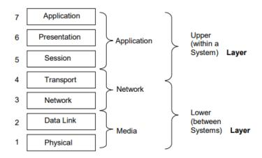
The OSI model is divided into two layers: upper layers and lower layers.
