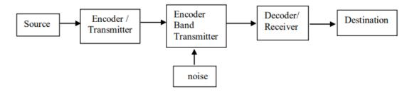
The communication system essentially consists of five parts:
