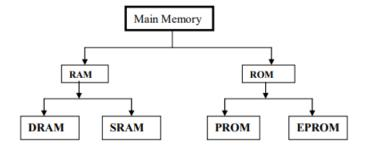
RAM(Random Access Memory): The Read and write memory (R/W memory) of a computer is called a RAM. The user can write information into RAM and read information from it. It is called random access since any memory location can be accessed in a random manner for reading and writing. The access time is the same for each memory location. Random
