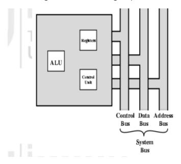
Arithmetic Logic Unit(ALU): The Arithmetic and Logic Unit is that part of the CPU that actually performs arithmetic and logical operations on data. It performs the basic arithmetic, logical operations specified by the instructions. Arithmetic operations includes addition, subtraction, multiplication, and division. Logical operations includes comparison, selection and merging of data. The CU, CPU registers and memory help in bringing the data into the ALU and then taking the results back.
