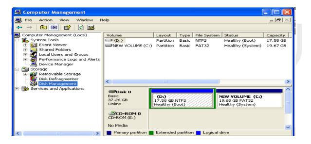
In Disk Management window, the upper section displays lists of all the partitions in the disk, and the bottom section contains the graphical representation of the drives in the computer.
